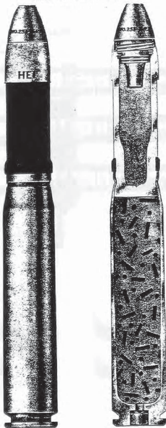
Figure 24 — CARTRIDGE, HE-I, Mk. I, w/FUZE, P. D., 253 Mk. II-III, 20-mm Guns, M1, AN-M2, M3, and Br. H.S./A/
