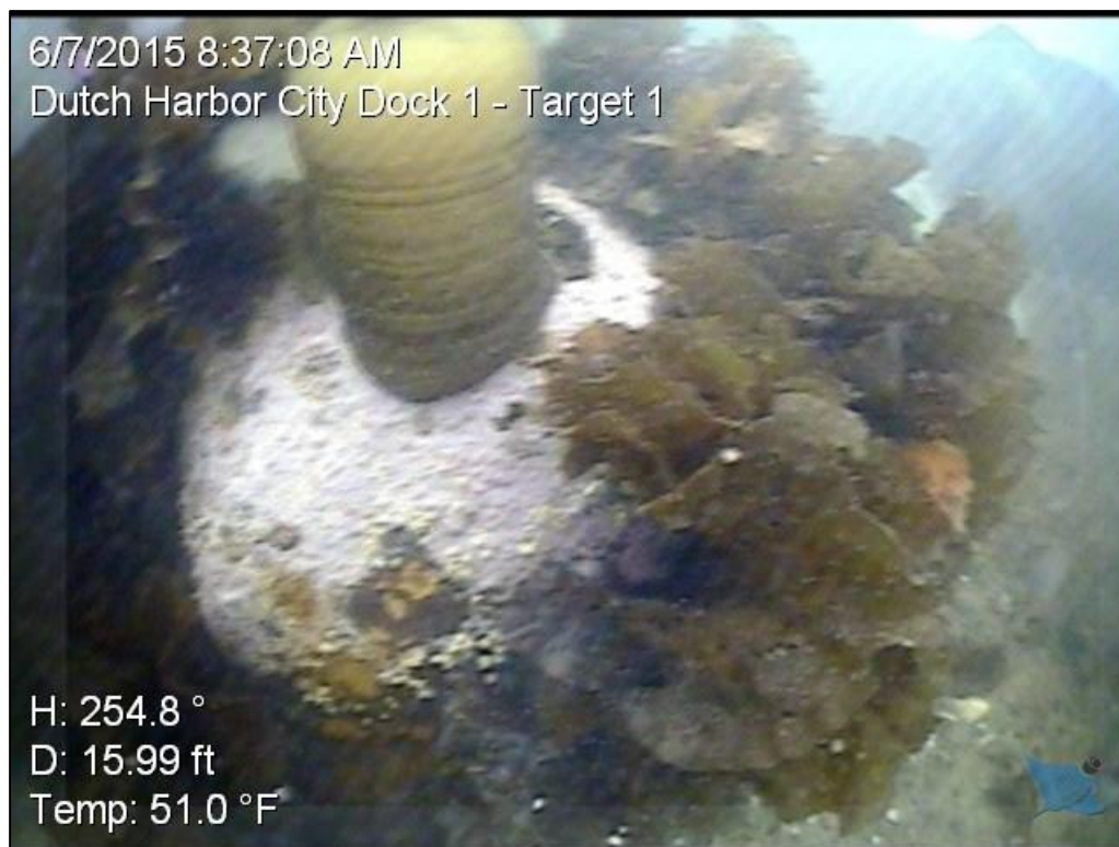
RI_ROV_DutchHarborDock1_Target_01. Nose of target, heavily overgrown with kelp and marine growth. However, bulbous nature of target is visible.
