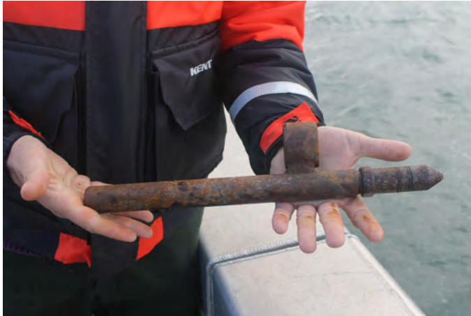
Figure 3-11a Test Shape – Mock 40-mm Shell
