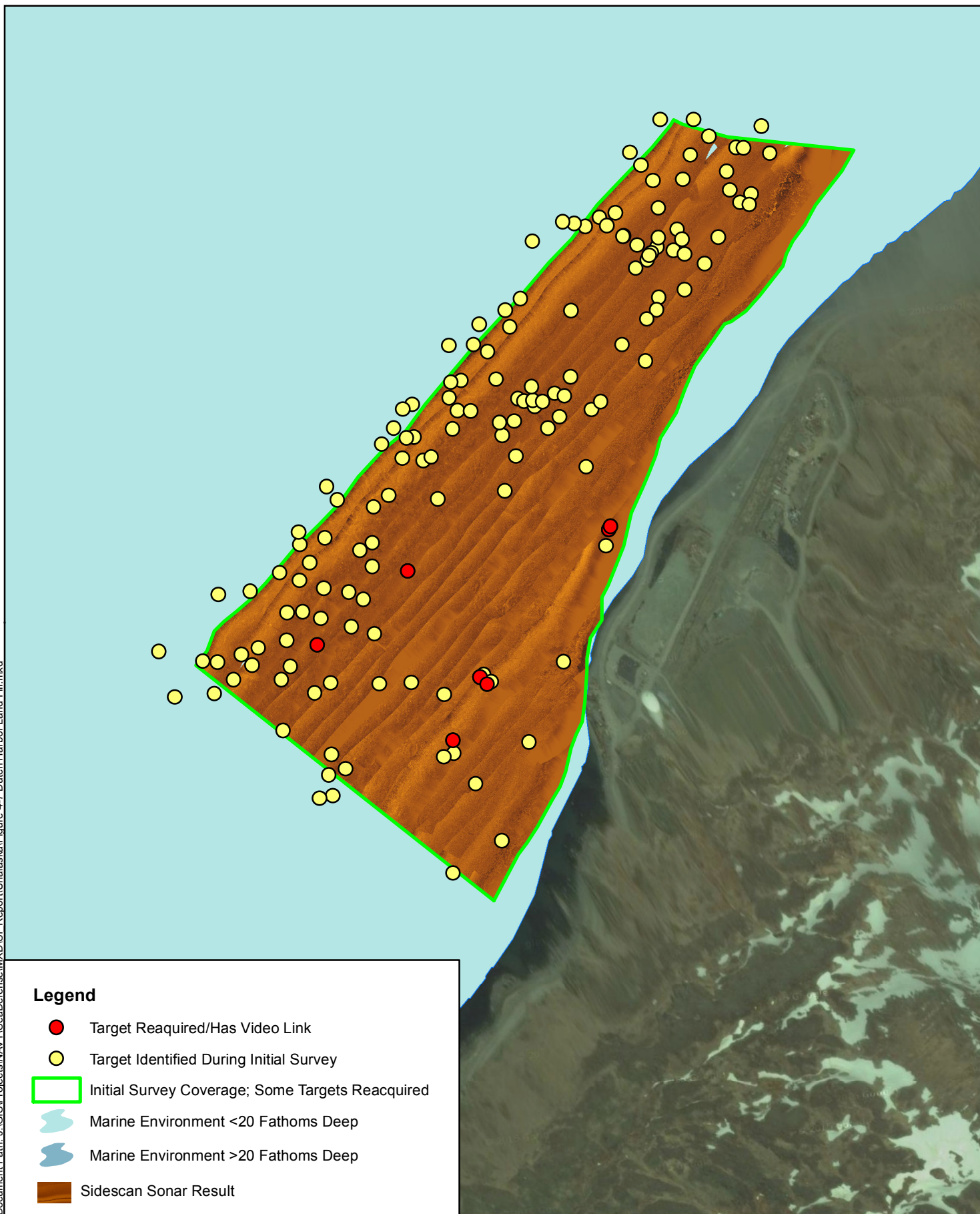
Figure 4-7 Seafloor Near Dutch Harbor Land Fill, Sidescan Sonar Results and Target Locations
