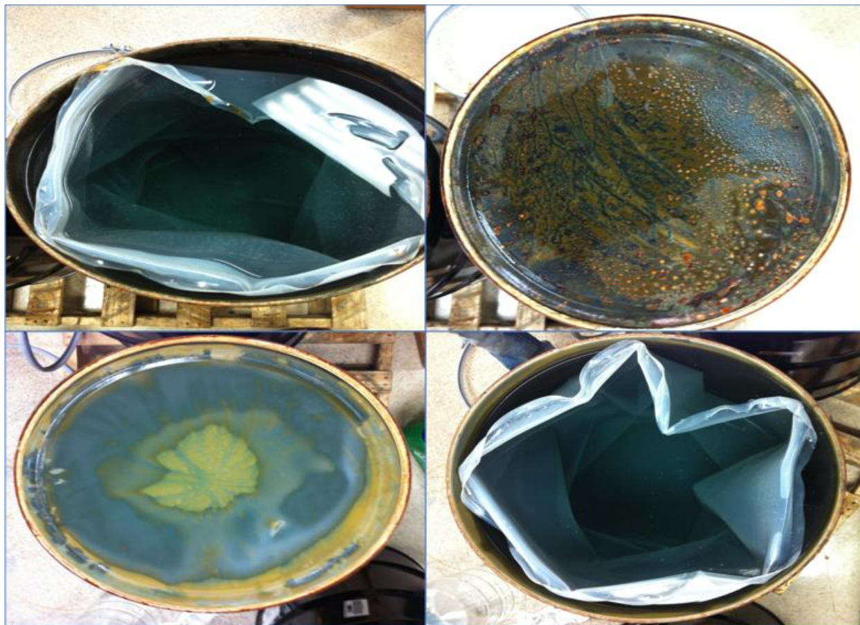
Figure 1: Iron Leaching out from the drums
