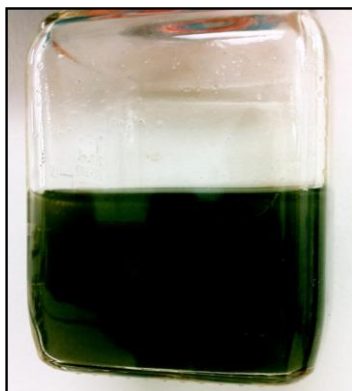
Figure 6a: GW aerated and pH raised to 10
