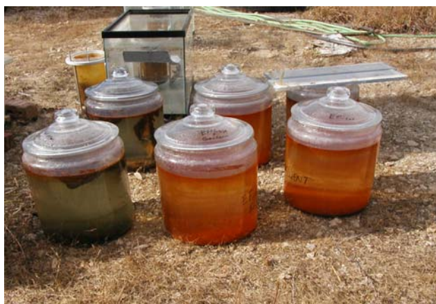
Figure 6. Batch Microbial Mat (left) and Bacteria (right) Treated Bioreactors
