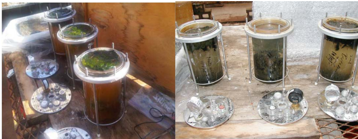
Figure 5. Greenhouse Tests: Multiple Batch Microbial Mat Bioreactors (Left =Day 1; Right = Day 3)
