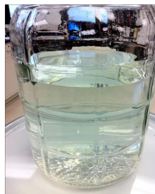
Figure 7: Final sample, aerated, pH raised to 10 and then filtered using sand filter7s
