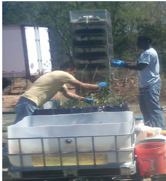
Figure 10 Microbial Mat Plate-and-shelf bioreactor operated in series with a CB1190 bioaugmented containerized constructed treatment wetland under ambient conditions.
