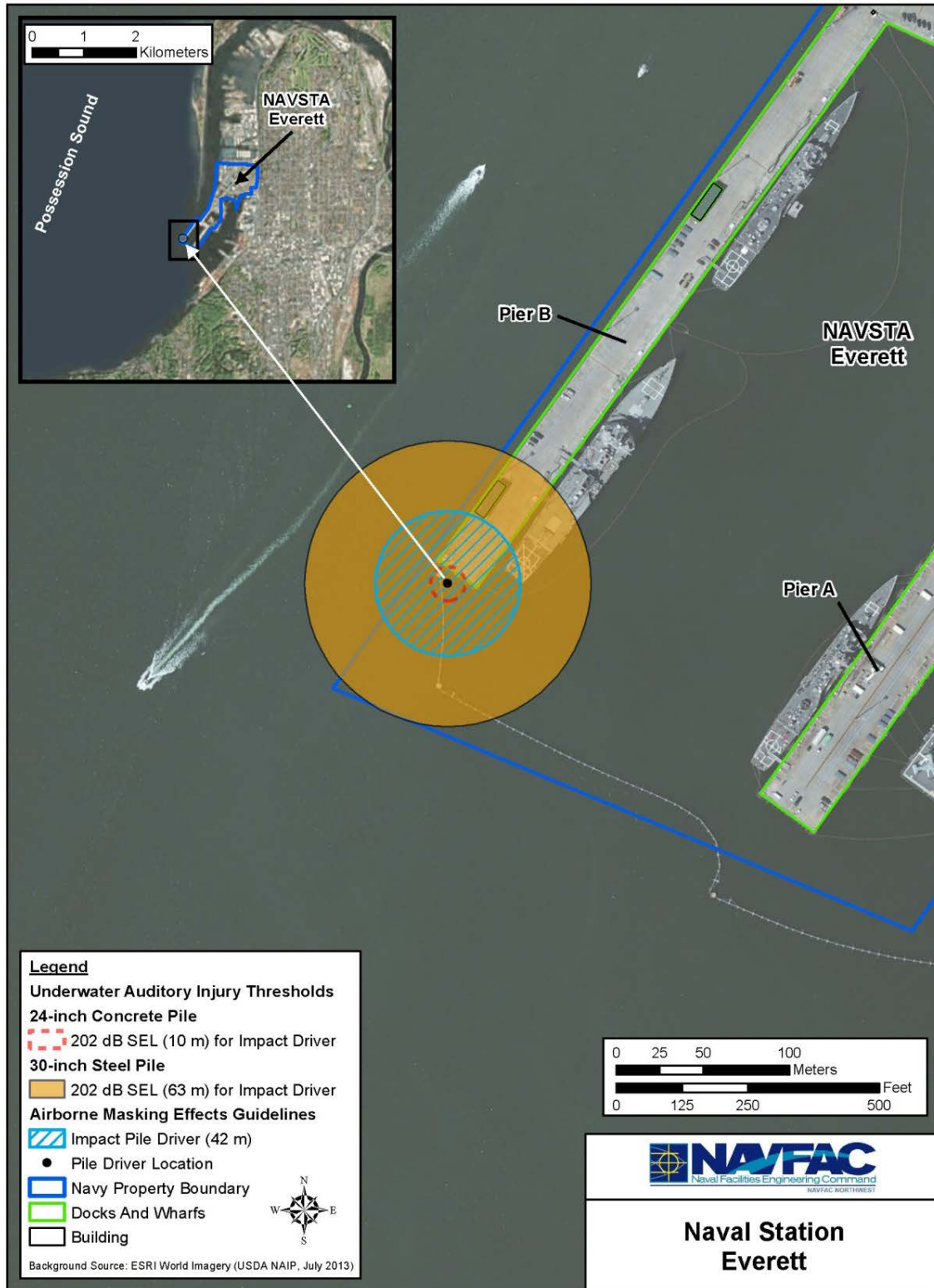
Figure 9-2. Representative Affected Areas for Pile Driving Noise for Marbled Murrelets at NAVSTA Everett
