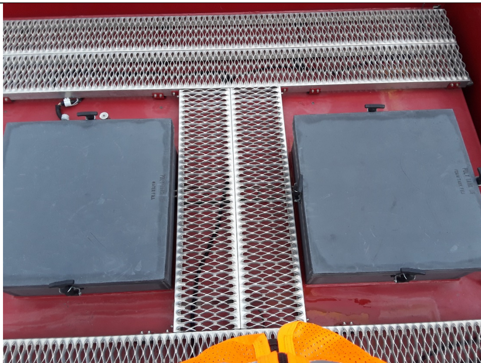
-Whidbey 37 water (left) and AFFF (right) tanks (2'x2' openings). Labeled Foam tank and Water tank.
