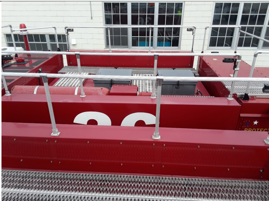
-Water (left) and AFFF (right) tank openings on Whidbey 36 from top of Whidbey 37 (Facing North).
