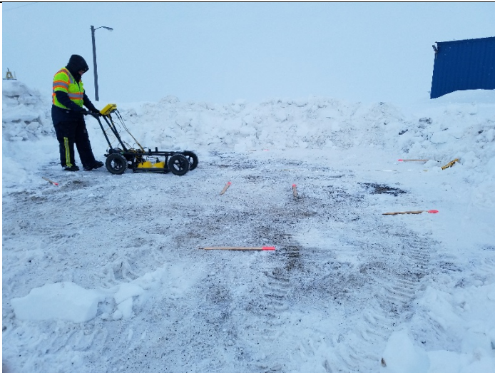
Performing GPR after clearing snow at Location 3 (Looking North) 08 March 2018
