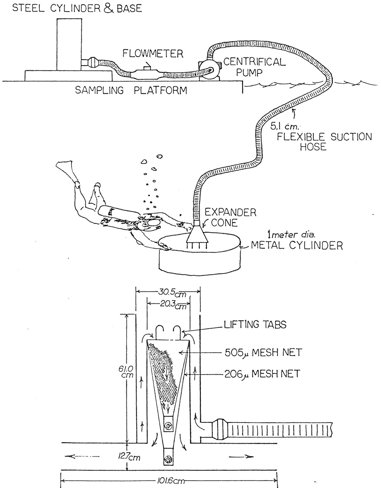
Fig. 8. Overall system design and construction detail of epibenthic pump sampling system.
