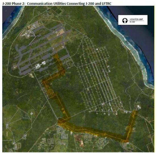
Project will install communication lines between J-200 and the LFTRC. Approximate path is highlighted; actual APE follows existing road and utility corridors within the shaded area.
