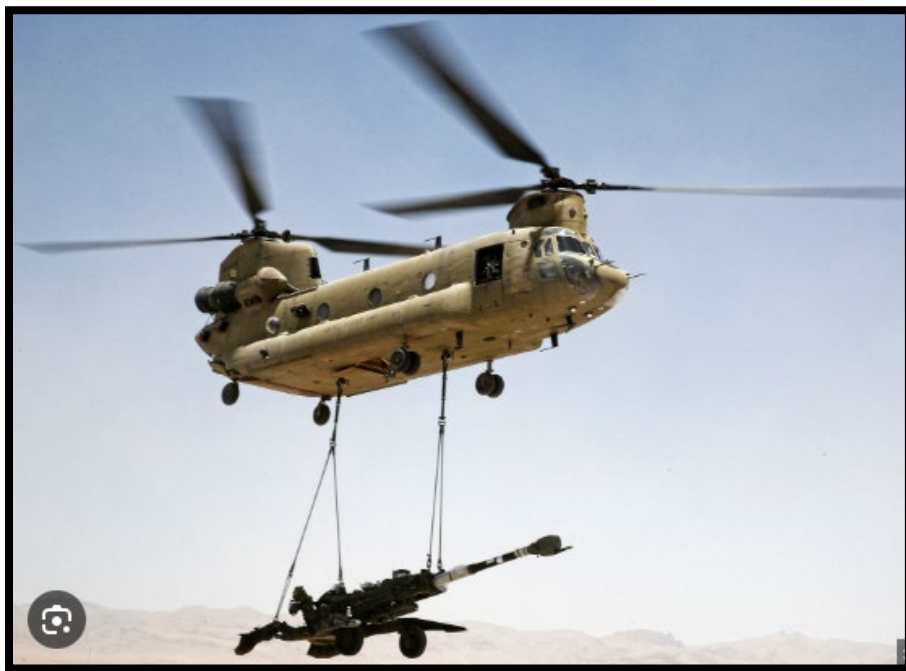
Figure A-18: Helicopter Sling Load of M777 Howitzer
