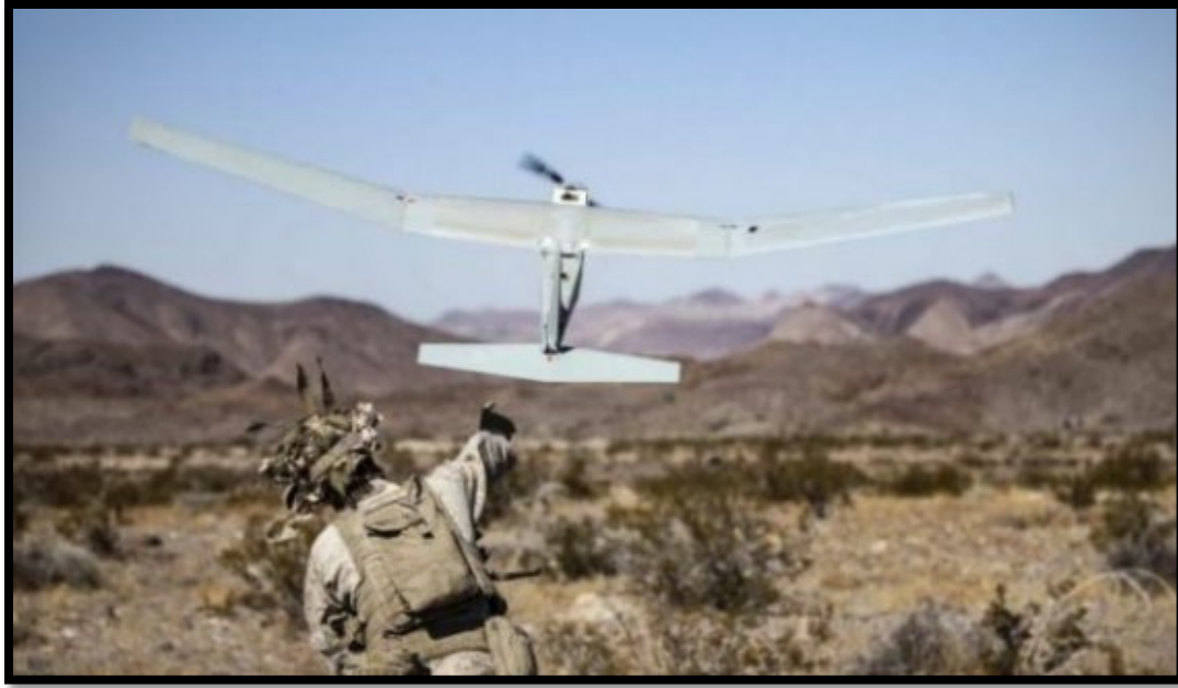
Figure A-10: Small Unmanned Aerial Vehicle Launch
