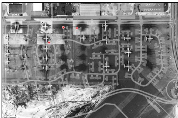
Figure 2: 1950's aerial photo overlain by future Onizuka Village housing development. Red asterisks (*) are locations of petroleum affected soil found in 2009.
