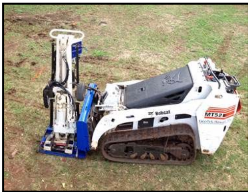
Figure 3: Track-Mounted Direct Push Technology Rig
