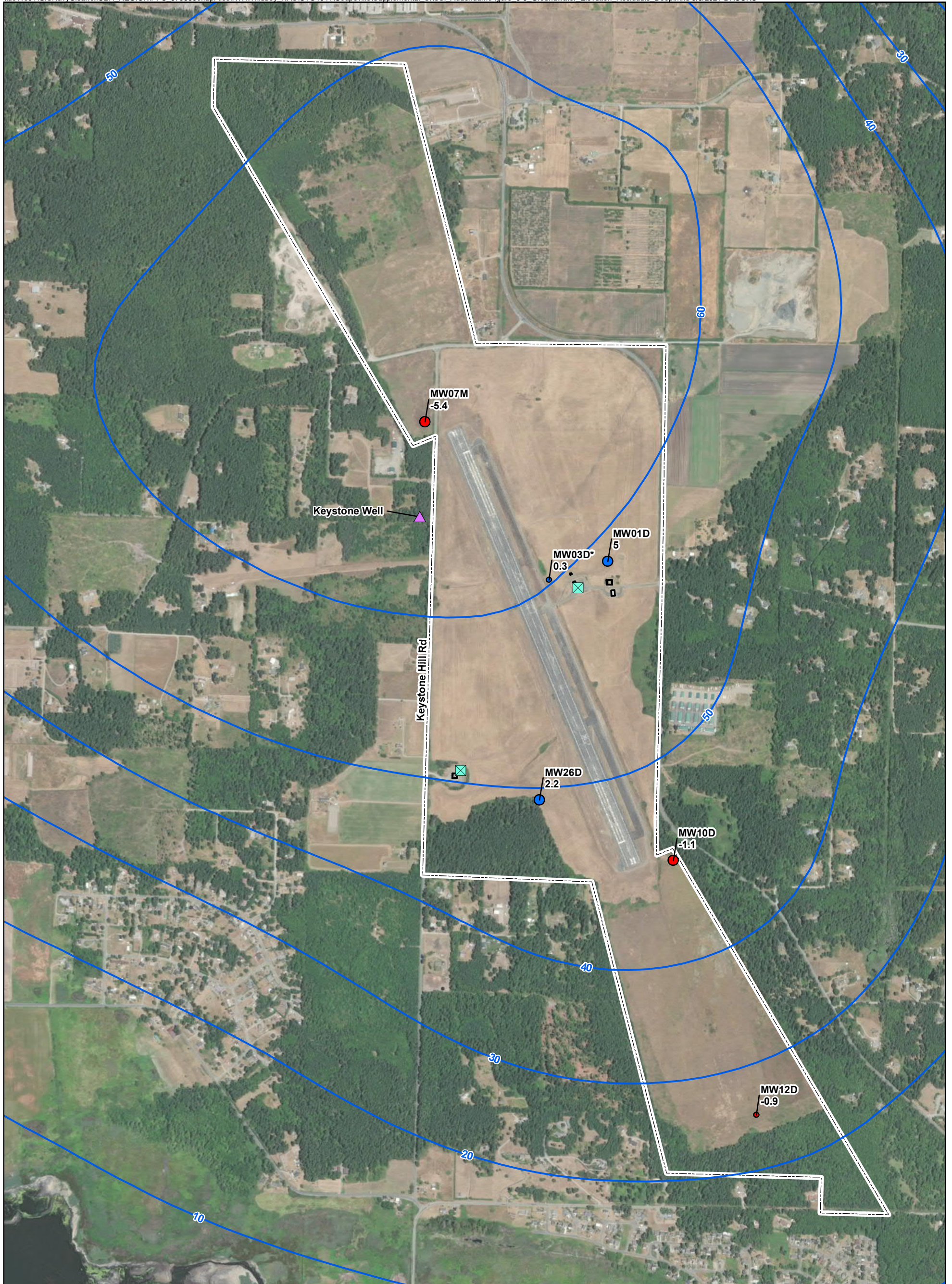
Figure 3-6 Simulated Steady-State Groundwater Elevation Contours and Residuals Deep Elevation Interval Naval Air Station Whidbey Island Coupeville, Washington
