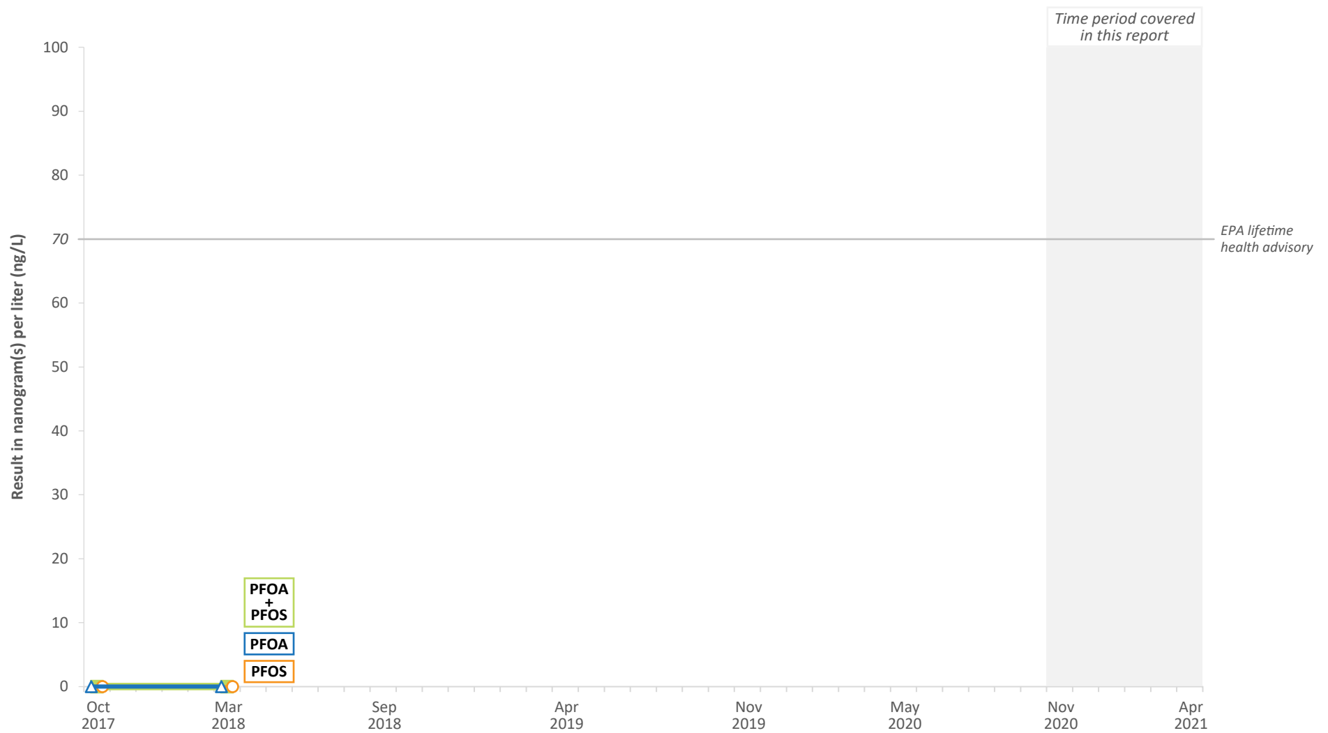
Figure A4-32. PFOS and PFOA in Drinking Water at Sample Location WI-AF-1RW11 Naval Air Station Whidbey Island Coupeville, Washington
