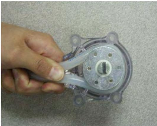
3. Turn rotor counterclockwise until tubing completely surrounds the rotor.
