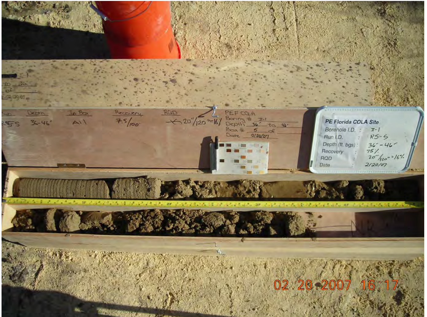
Example of sonic soil cores - overall box photograph with box close ups (left and right sides).
