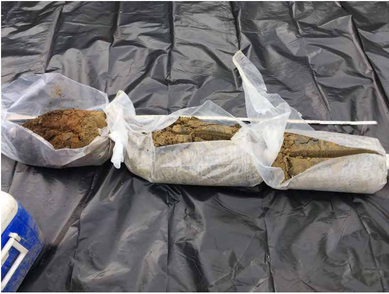
Photo 3. Example of sample recovery from 0-210 cm below ground surface. Top of core sample is at left. Note distinct color change from A to B Horizons.
