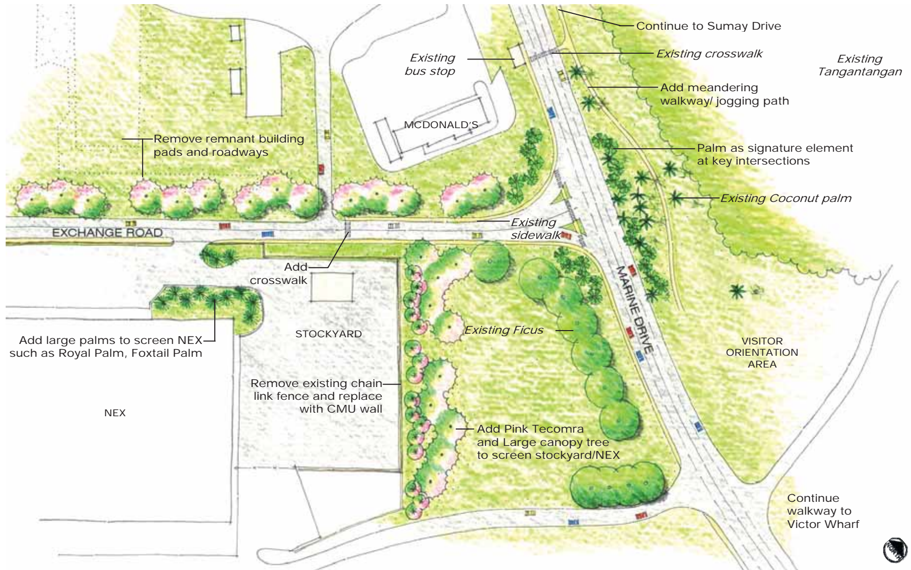
Figure 7.16. Project #6 Exchange Road Improvements: Segment C - NEX/Commissary to Marine Drive
